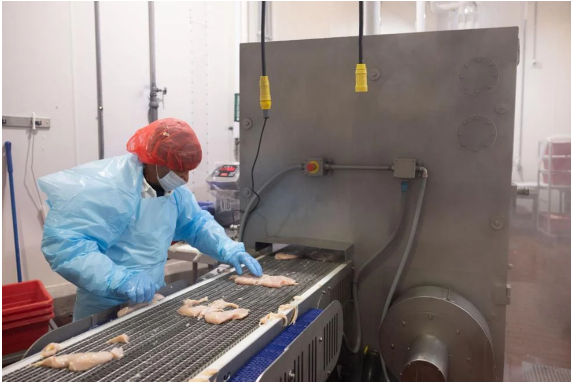
A Ukrop's employee separates breasts from trim after it is cut by pressurized jets of water at the Ukrop's Kitchen in Chesterfield.
